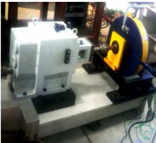
Engine Dynamometer for Performance & Endurance tests on small portable Engines & Agricultural Diesel & Kerosene Engine.
