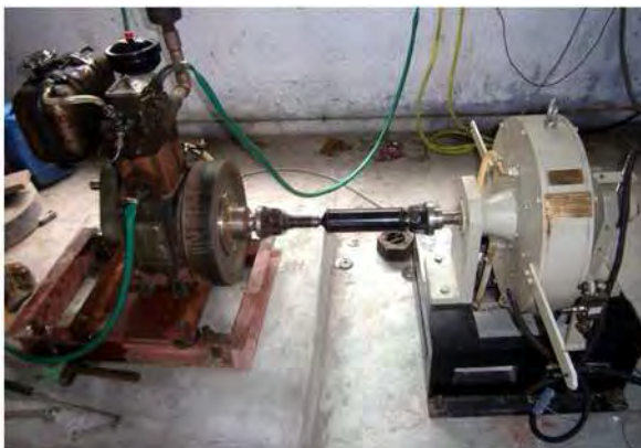
Engine Dynamometer for Performance & Endurance tests on small portable Engines & Agricultural Diesel & Kerosene Engine.
